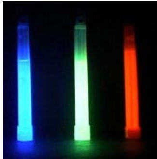
Commercially available light sticks contain a solution in a glass vial. When the vial is broken, a second solution mixes with the first and light (chemiluminescence) is generated. Different dyes give off different colors when they are caused to fluoresce by the light of the chemiluminescent reaction. (Photo: American Chemical Society)
