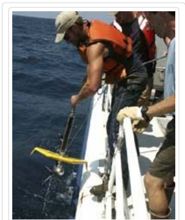
Deployment of the side scan sonar tow vehicle, also called a 'fish'. (Photo: NOAA)
